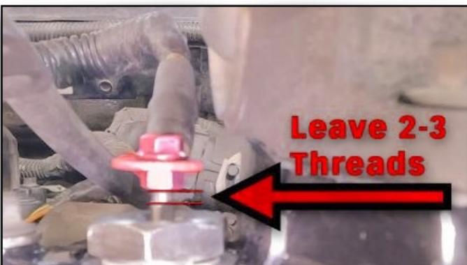
12V cable should be sandwiched in-between both nuts, away from metal contact.
