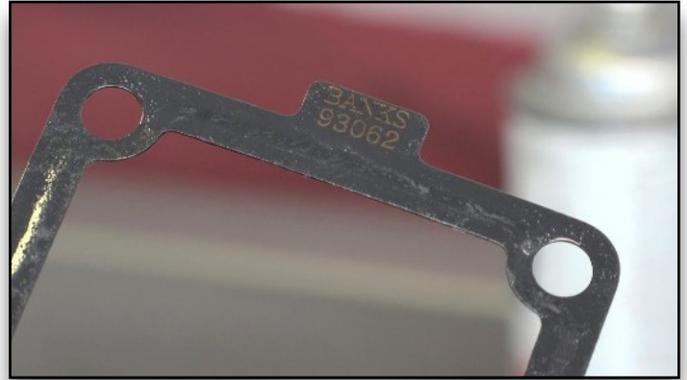
Side that says Banks, should be the side with the adhesive. Let it sit for about 3 min for the glue to tack up.
