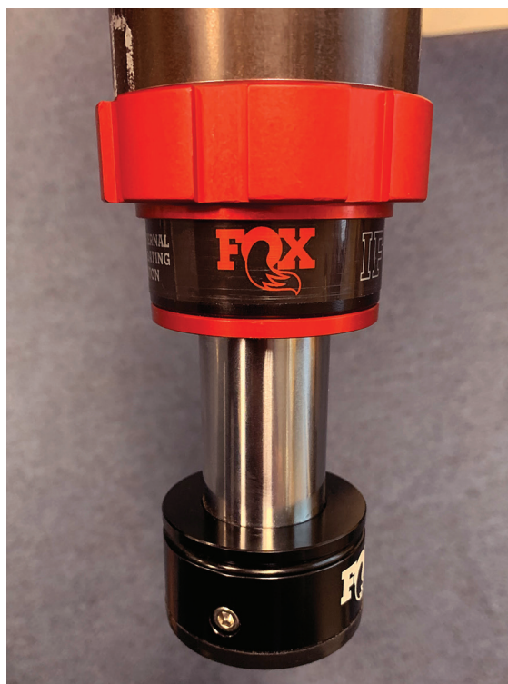
Figure 4: Lock ring installed
