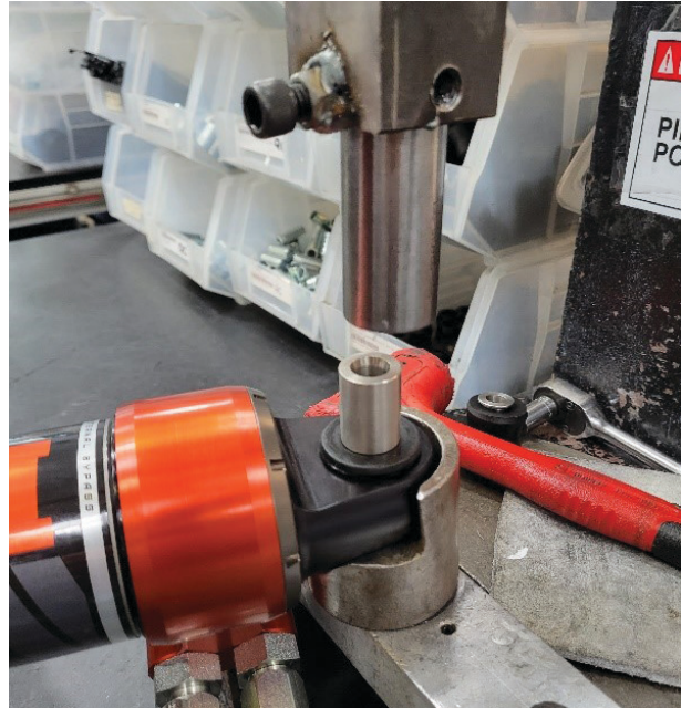
Fig. 8: Installed bushing and spacers in upper eyelet.
