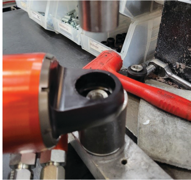
Fig. 4: Bushing and spacers are pressed out.
