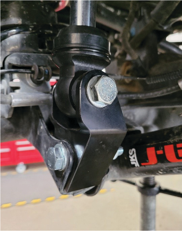
Fig. 9: Installed relocation block.
