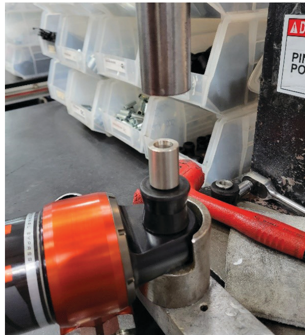
Fig. 6: Align the bushing and spacer with the eyelet.
