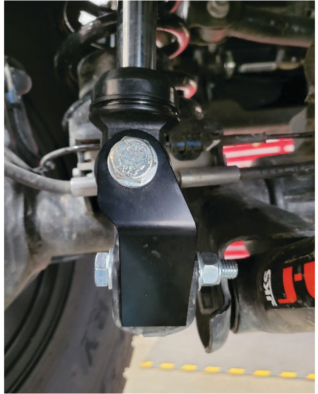
Fig. 10: Installed relocation block.
