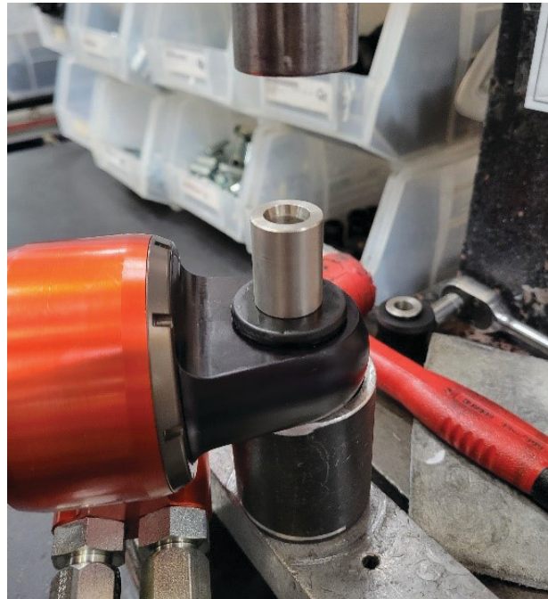
Fig. 2: Shock eyelet is aligned with the spare tubing and press.
