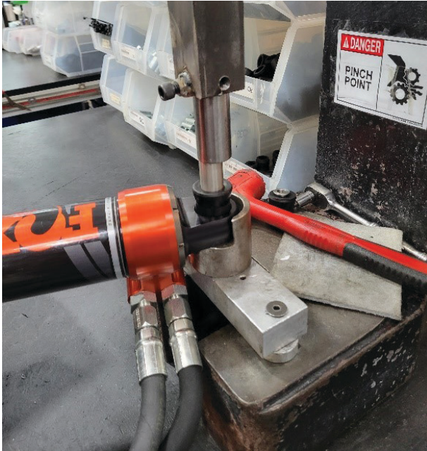
Fig. 7: Press the bushing and spacers.
