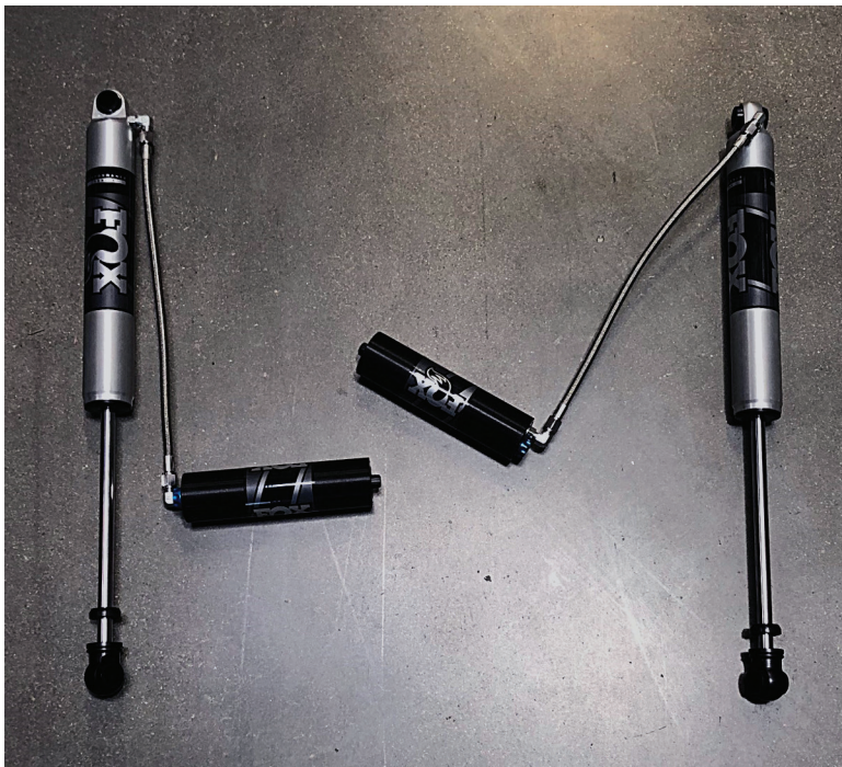
Figure 12: Rear left (L) and right (R) Performance Series shocks
