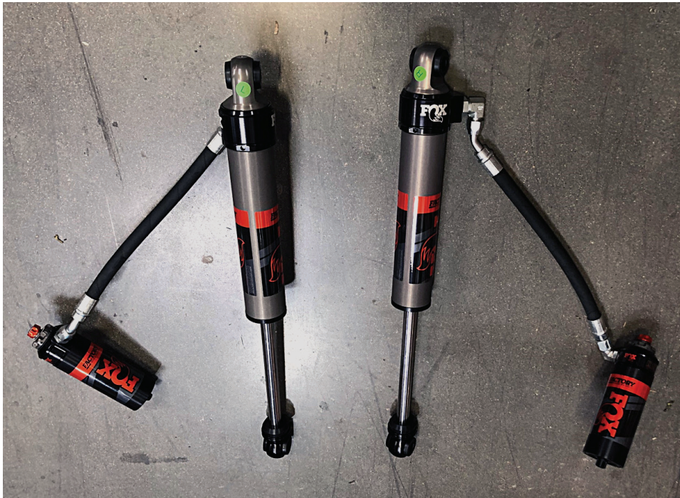
Figure 11: Rear left (L) and right (R) Factory Race shocks
