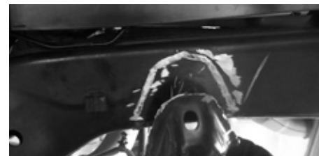
Fig. 3: Rear Factory bump stop bracket removed
