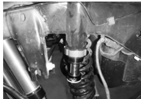
Fig. 7: Rear lock ring installed
