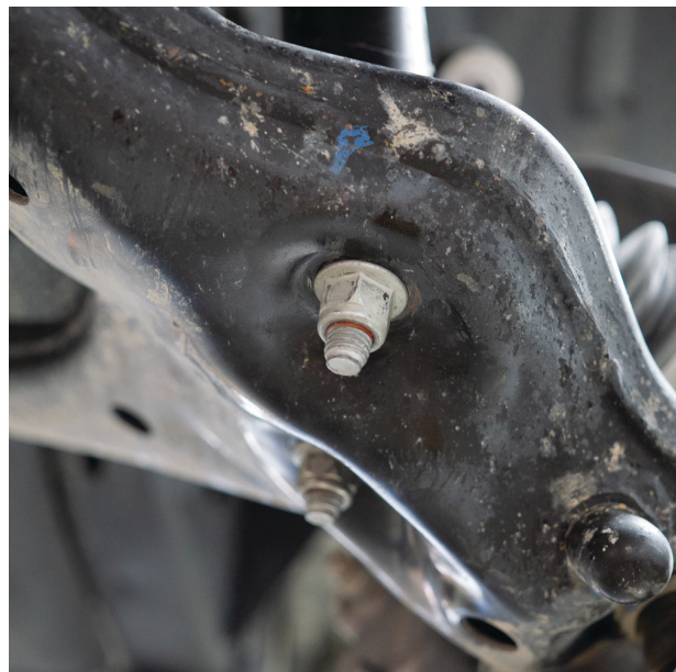
Fig. 7: Remove the bar-pin bolts.
