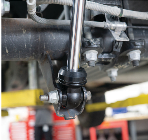
Fig. 19: Install the lower shock bolt.
