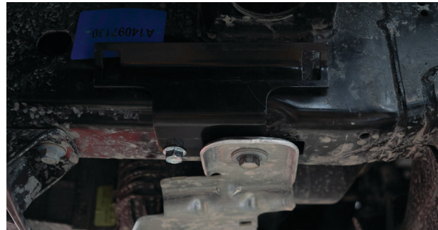
Fig. 9: Install the reservoir bracket.
