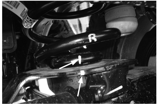
Mark spring location in reference to upper and lower spring seat. Sample of passenger's (right) side shown.
