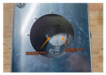
02. Install the pump onto the strainer basket inside the tank.
