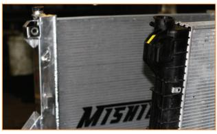
2. Transfer OEM rubber bushings/isolators to the Mishimoto radiator.
