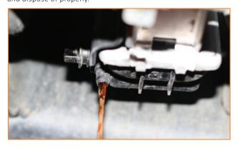
2. Remove the plastic clips holding the front air dams in place.
