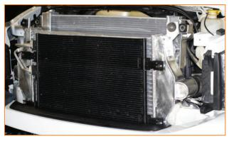
7. Reinstall the OEM upper radiator support using the (4) 1/2" head bolts.
