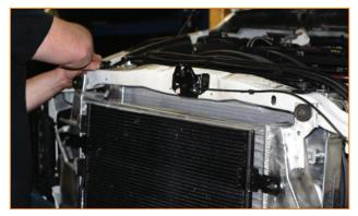
**8.** Reinstall the intercooler with the (2) OEM 10mm upper intercooler mounting bolts.
