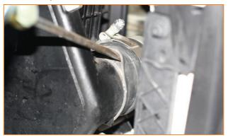
6. Remove the (2) 10mm head upper intercooler mounting bolts.
