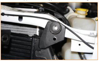
7. Lift intercooler with an up and outward motion to remove.
