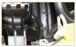
**16.** If your vehicle has a bolt attaching the intake system to the fan shroud, remove this and then lift up on the shroud to remove.
