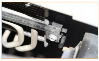
3. Slide the OEM fan shroud onto the back of the Mishimoto radiator.
