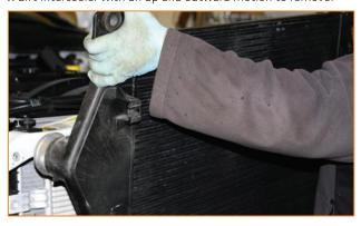
8. Pull couplers off the inlet and outlet end tanks of the intercooler.
