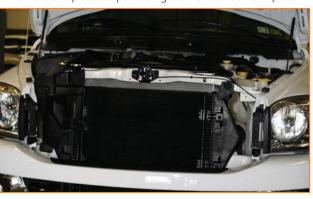
3. Remove the (4) 1/2" head bolts which hold the A/C condenser to the intercooler. Lift A/C condenser out and hang off to the side. **NOTE:** Do not disconnect the A/C lines. If lines are disconnected, the A/C system must be recharged.
