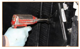
4. Loosen the (2) 11mm head T-bolts on the intercooler end tanks.
