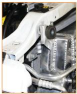
**10**. Remove the (2) 10mm bolts holding the radiator to the upper radiator support from the backside.
