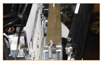
6. Reinstall the A/C condenser with the (4) 1/2" head bolts.
