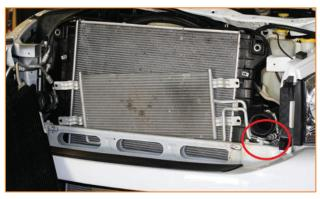
**18.** Remove the (2) 1/2" head bolts holding the Power Steering cooler onto the radiator and allow to hang once removed.
