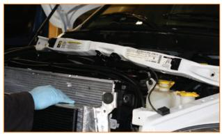
**12.** Remove the (2) 1/2" head transmission cooler bolts. Pull up on the transmission cooler to separate from the radiator. Lean the transmission cooler forward.
