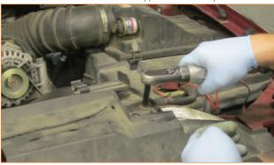
5. Remove three 8mm bolts for the coolant overflow container.
