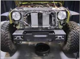
A thermocouple was mounted in the front grille with no obstructions so that ambient air temperatures could be measured.
