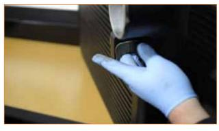
**3.** Place the Mishimoto intercooler into position. Be sure the grommets seat properly in the cross bar that supports the radiator.
