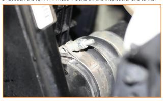
4. Loosen couplers from intercooler with a screwdriver.
