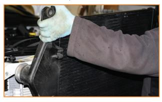
7. Remove the OEM intercooler coupler from the charge piping.
