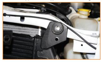
6. Lift intercooler with an up and outward motion to remove
