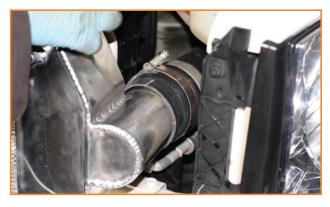
4. Reinstall the (2) OEM 10mm upper intercooler mounting bolts and tighten OEM T-bolt clamps.
