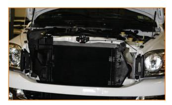
2. Remove the (4) 1/2" head bolts which hold the A/C condenser to the intercooler. Lift A/C condenser out and hang off to the side.
