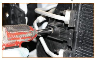
3. Loosen the (2) 11mm head T-bolts on the intercooler end tanks.
