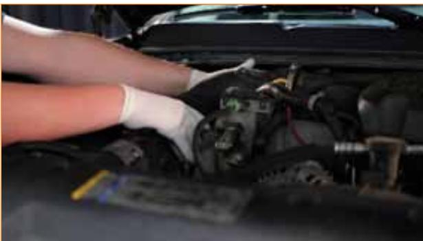
4. Remove the airbox from the engine bay.
