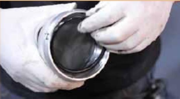
3. Install the lower cold-side pipe to the intercooler. Loosely place a clamp over the pipe but do not tighten it yet.
