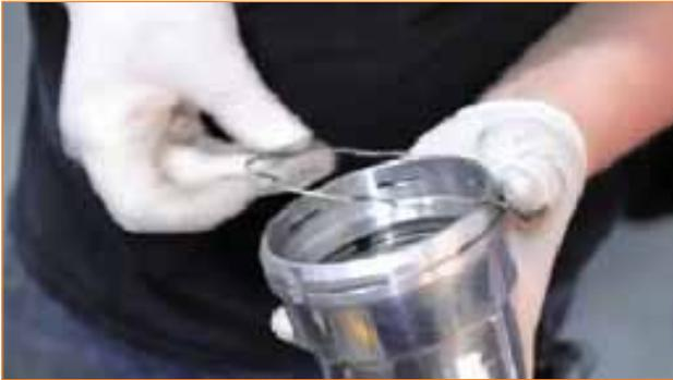
2. Attach the provided O-ring gaskets to the Mishimoto intercooler pipes. Use a little bit of oil on the O-rings to ensure a proper seal, and to allow the pipe to slide on easily.
