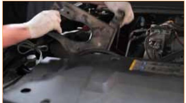
7. Remove the two retaining clips that connect the cold-side intercooler pipe to the intake manifold and intercooler.
