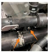
11. Using an 8mm socket, remove the bolt holding the ground strap and tuck the strap on top of the cross member.
