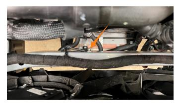
12. Using a 15mm socket, loosen the 2 rear bolts and completely remove the rest of the bolts. Remove the front skid plate/splash guard. Both the plastic splash guard and metal skid plate are shown below. (Image on top right)
