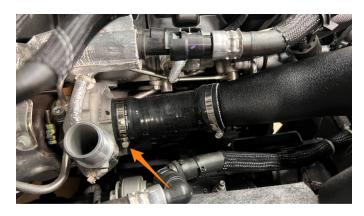
9. Using an 8mm socket, remove the bolt securing the airbox in place (left image below). Remove the intake air temperature sensor (right image below) from the intake pipe by rotating it about ¼ turn counterclockwise and pulling out. Remove the airbox from the vehicle.
