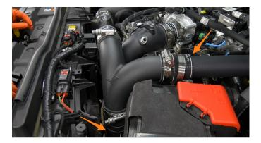
**33.** Install the assembly from steps 27/28 on the passenger-side of the engine, being sure to get the boot onto the turbo outlet and the other end of the pipe into the other side of the "Y" from the previous step.
