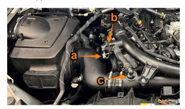
3. Using an 8mm socket, remove the three bolts securing the hot-side intercooler pipe to the air intake (a). Using a 7mm socket, loosen the hose clamp (b). Release the quick disconnect clip (c) and lift the passenger-side hot-side intercooler piping assembly out of the yehicle.
