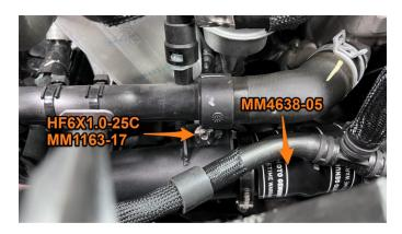
25. Install boot 6 onto the throttle body and slide 2x 92mm clamps over the boot. Insert the bottom of cold-side pipe 2 into the boot from the previous step then rotate the top into the boot on the throttle body. After ensuring proper alignment, use a 10mm socket to tighten all the clamps on the cold-side pipes. Using a 10mm socket, install the stock sensor into port (a) using the provided 6mm bolt, HF6X1.0-20A. (Image on next page)
