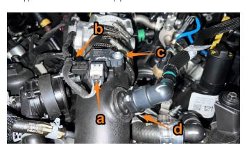
7. Using a 7mm socket, loosen hose clamps (a) and (b). Using an 8mm socket, remove bolt (c). Remove the intake pipe.
