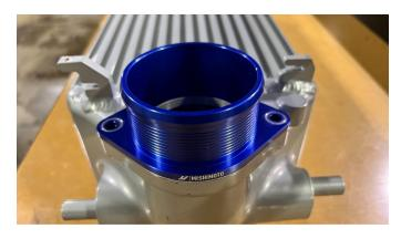
19. Remove the blue quick disconnect adapter and boot from the Mishimoto high-mount intercooler. Skip to step 21.
