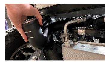
22. Once in position, slide the boots onto the intercooler adapters. If you're using a stock intercooler, the pipes should be inserted such that the edge of the boot is lined up with the 2nd white line from the end of the pipe and the 1st line if using a Mishimoto stock-location intercooler. Position the clamps on the boots and loosely tighten them. Skip to step 24.
