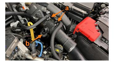
6. Unplug connector (a) and use a trim clip tool to remove tree clip (b). Using a T25 Torx, remove screw (c) and remove the sensor from the upper cold-side intercooler pipe.
