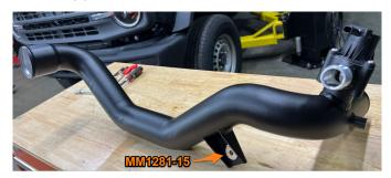
13. Using the provided clamps and turbo boot, install the Mishimoto hot-side intercooler pipe. Do not tighten the clamps, this will be done later. Reconnect the bypass valve hose and electrical harness. (MM4623-01, MM1533-66, and MM1533-79)
