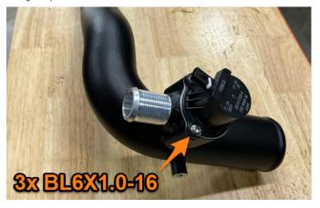
12. Install the provided grommet onto the Mishimoto hot-side intercooler pipe. (MM1281-15)
