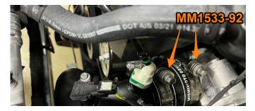
17. Connect the Mishimoto hot and cold-side intercooler pipes to the Mishimoto high-mount intercooler using the provided boots and clamps. (2x MM4634-01, and 4x MM1533-92)
