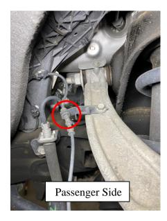
E. Use a 21mm deep socket to remove nut from tie rod end. Then use a tie rod separator to remove the tie rod from the knuckle.
