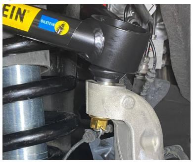
W. Reinstall the tie rod end to the spindle using a 21mm wrench and 10mm wrench. Then using a 10mm wrench, reinstall the brake line bracket and ABS line bracket to the rear of the spindle.
