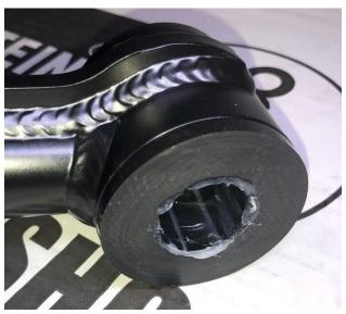
O. Press the steel sleeves into the bushings and apply more grease to outside faces of the bushings and sleeves.
