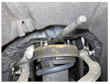
Remove the shock for access to the upper control arm bolts. Using a 21mm socket and 21mm wrench, remove the upper control arms.
