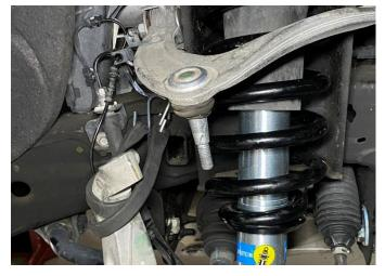
H. Using a 15mm socket/wrench, remove the two bolts securing the shock to the lower control arm.
