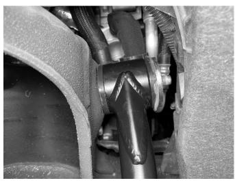
R. Apply non-permanent thread locker to the UCA bolts and install the flanged nuts. Torque bolts to 122 Nm (90 ft. lbs.) Wipe off the excess grease.
