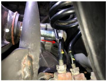
H. For 2017+ Titan, on left (driver) side only: Locate the two hoses mounted to a bracket rearward of the UCA. Use a 10mm socket to remove the two bolts securing the bracket to the frame (the first bolt is circled below, the second is on the inside of the frame rail) and remove the bracket from the hoses at four clip points (arrows below). This will allow for removal of the rear UCA pivot bolt by carefully moving the hoses until they clear the bolt.
