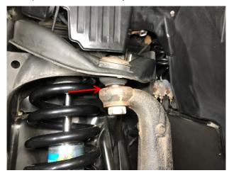
E. Remove the ball joint nut and remove the spindle from the UCA. Secure the spindle using a bungee cord or bailing wire. Be careful to avoid tension on the brake line and ABS line.
