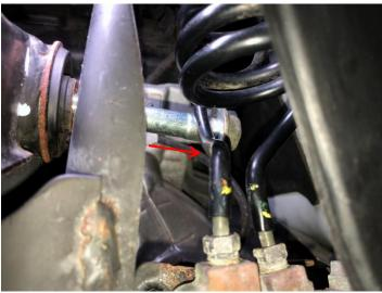
H. Carefully remove the remaining UCA bolts. The UCA can now be removed. Save the UCA bolts and nuts as they will be reused later.
