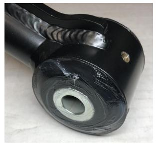
M. Install the 4 provided 90° zerk fittings into the threaded holes on the top of each bushing eye-ring ensuring they face outboard for easy access during service.
