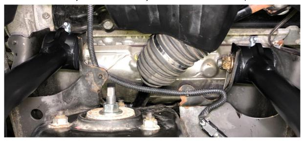
O. Install UCA ball joint on the spindle and secure using castle nut provided. Using 21mm socket, torque castle nut to 78.5 Nm (58 ft.lbs.). Continue to tighten the castle nut to the next available slot (no more than 60°). Never back off the slotted nut to achieve alignment with the hole in the stud. Install the cotter pin.
