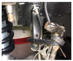
F. Using a 19mm socket and 19mm wrench, remove the nuts from both UCA pivot bolts. Leave the bolts in place at this time. Note that both UCA pivot bolts are facing forward toward the front of the vehicle with the head of the bolts on the rear side of the vehicle.
