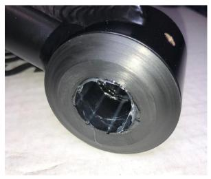
L. Press the steel sleeves into the bushings and apply more grease to outside faces of all bushings and sleeves.
