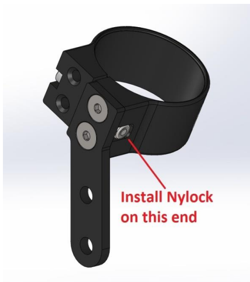
Figures 6 & 7 - Front and Back View of Vehicle Right Side Assembly
