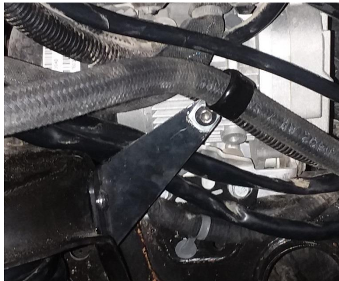
Figure 31 – Right Reservoir Hose Installed
