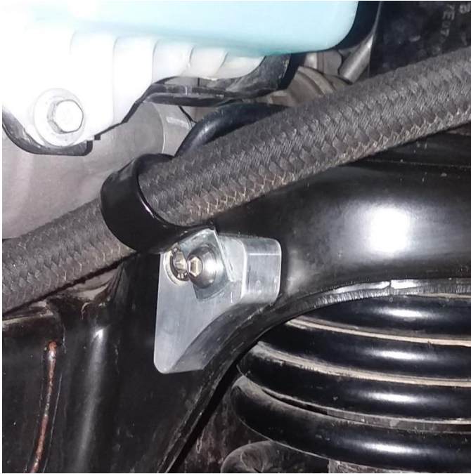
Figure 29 – Left Reservoir Hose Installed
