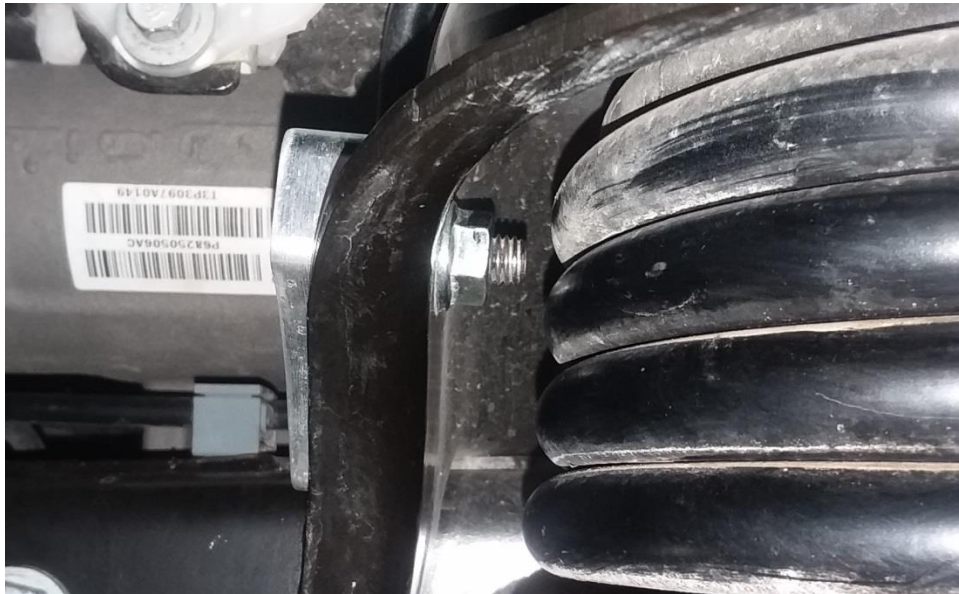
Figure 11 – Vehicle Left Side Serrated Flange Nut Installed
