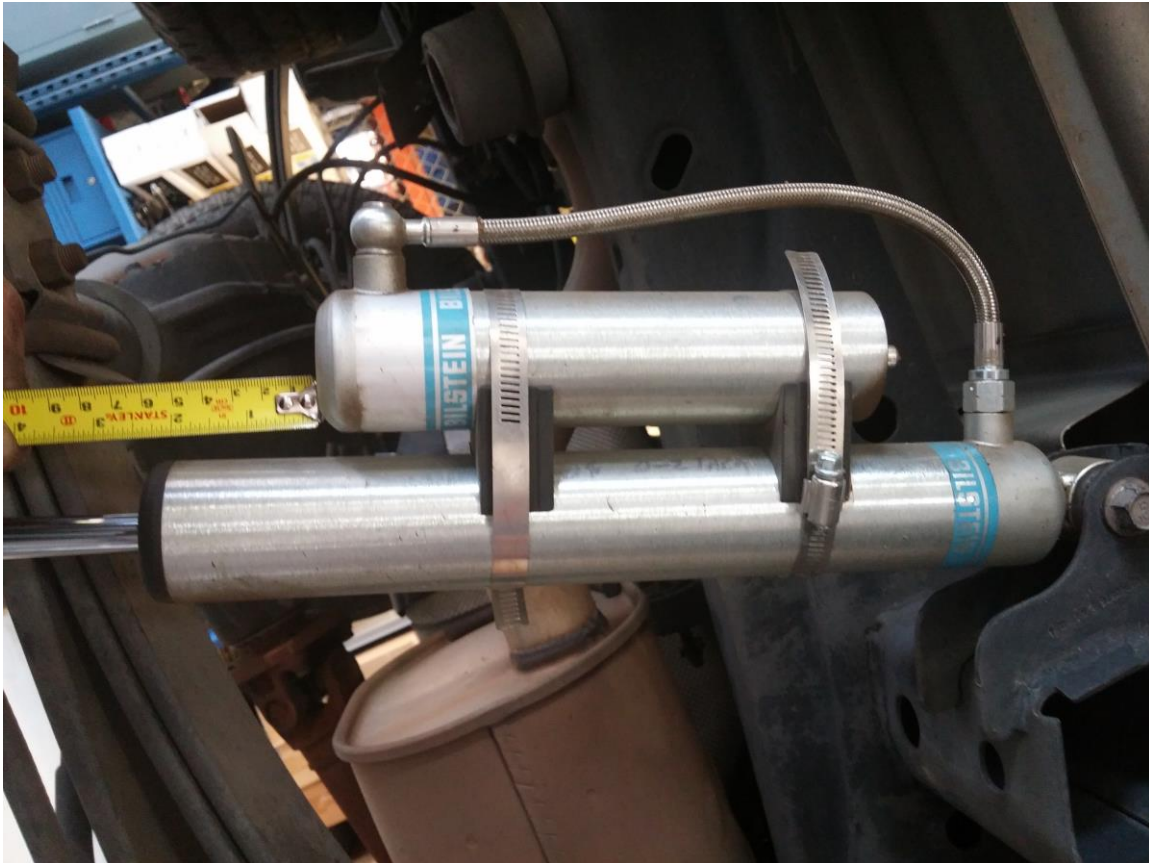
Figure 2. Reservoir placement in relation to end of main tube. Reservoir end should be about 2.25"-2.5" from end of main tube.
