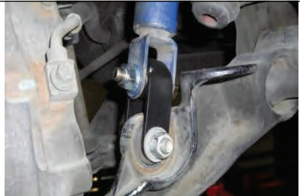
66-3000 Install front lower shock extensions and hardware
