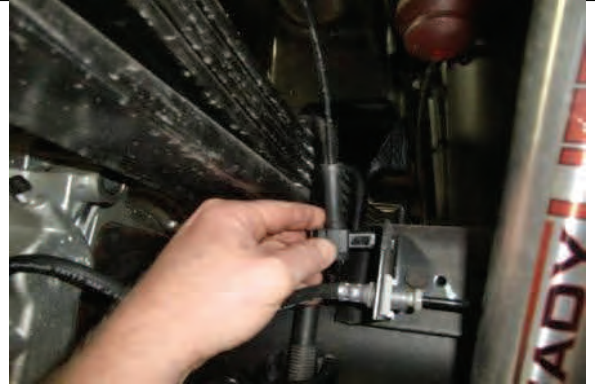
Release ABS clip from bracket on axle.
