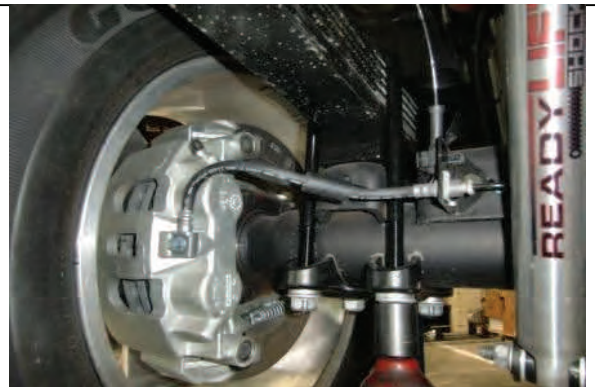
Torque U-bolts with vehicle on ground and re-clip ABS wire
