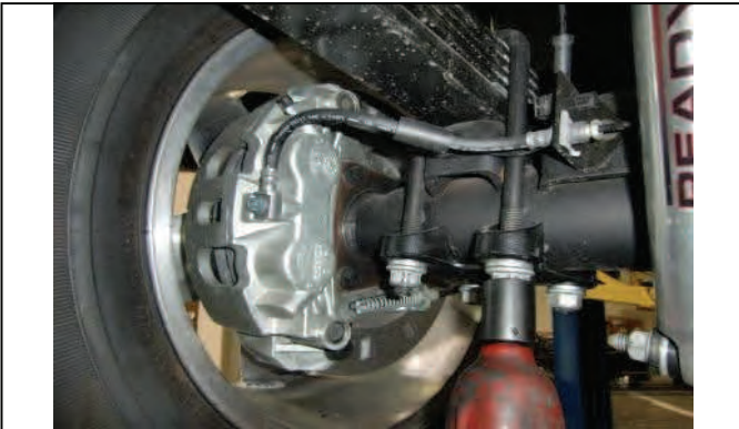
Support axle and remove U-bolt hardware and axle bracket
