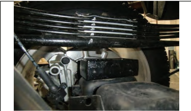
Note slight taper on block, shorter end towards front of truck
