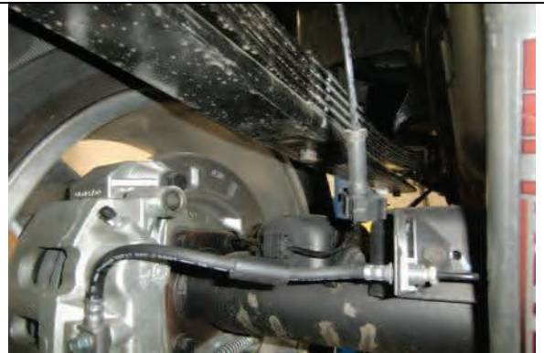
Remove U-bolts and lower axle to allow lift block positioning
