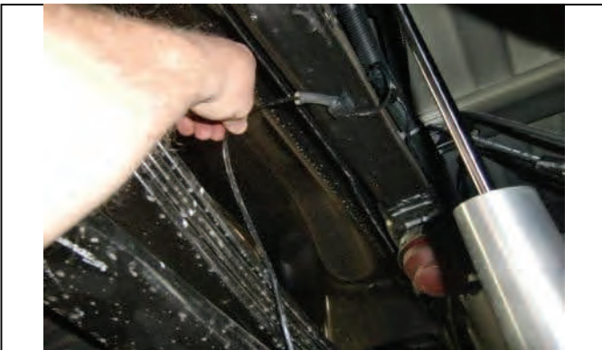
Slide ABS wire clip at frame up to gain slack to avoid damage
