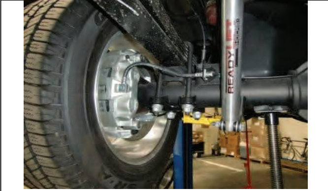
Raise and support vehicle on level ground and support frame.
