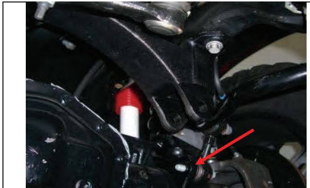
(05-10) Re-attach and tighten sway bar end links.
