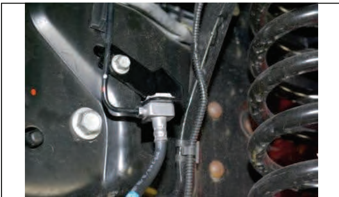
Reinstall block into bracket with retaining clip.
