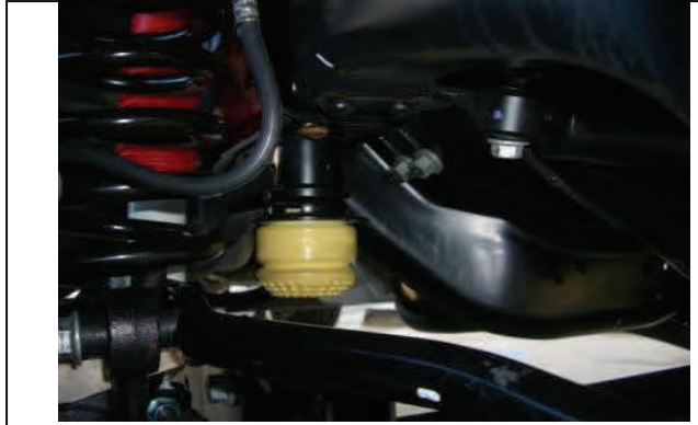
Assemble bump stop bracket to extension and reinstall.
