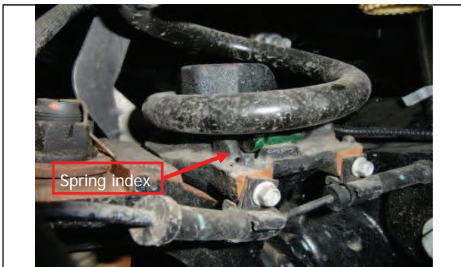
Raise axle and clock coil spring on lower mount as shown .
