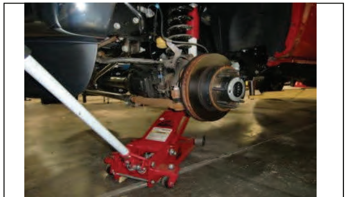
Support front axle with floor jack(s).
