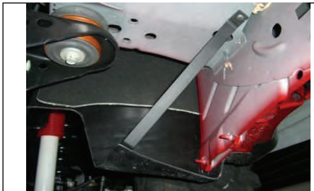
(05-10) Install fender liner strap to clear larger wheel/tires
