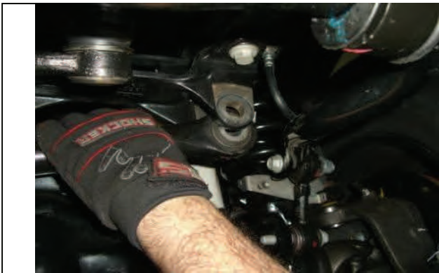
Re-attach trac bar to frame mount and torque to spec.
