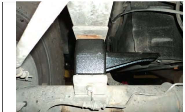
Remove OE axle block and replace w/ new lift block.
