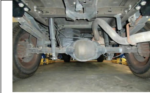
Place vehicle on level ground and lift and support by frame
