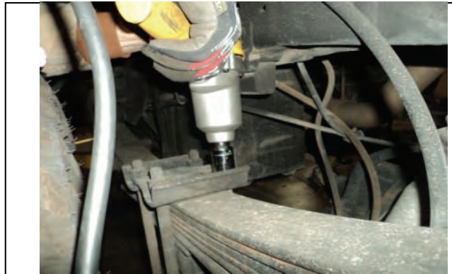
Remove u-bolt nuts on top of leaf spring plate
