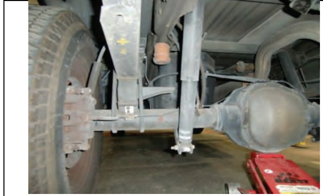
Also support axle by differential
