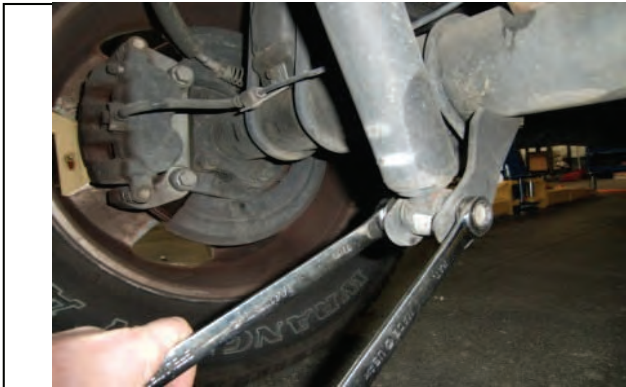
Disconnect lower shock mounting hardware.
