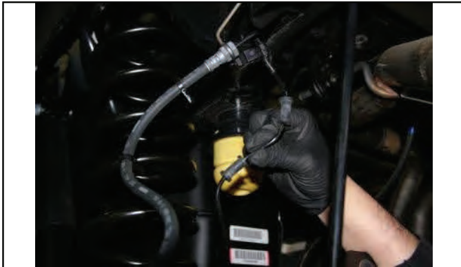
Disconnect ABS lines to avoid damage during installation.
