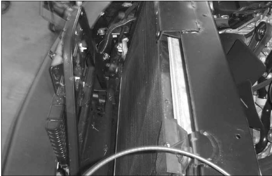
Figure 2.8 Upper Intercooler (CAC) Attachment Bolt.
