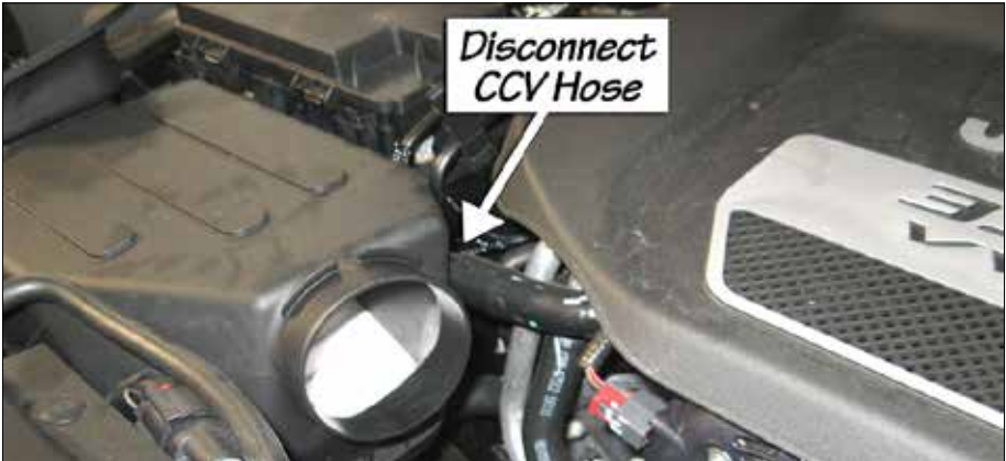
Figure 3- Disconnect CCV hose from intake housing
