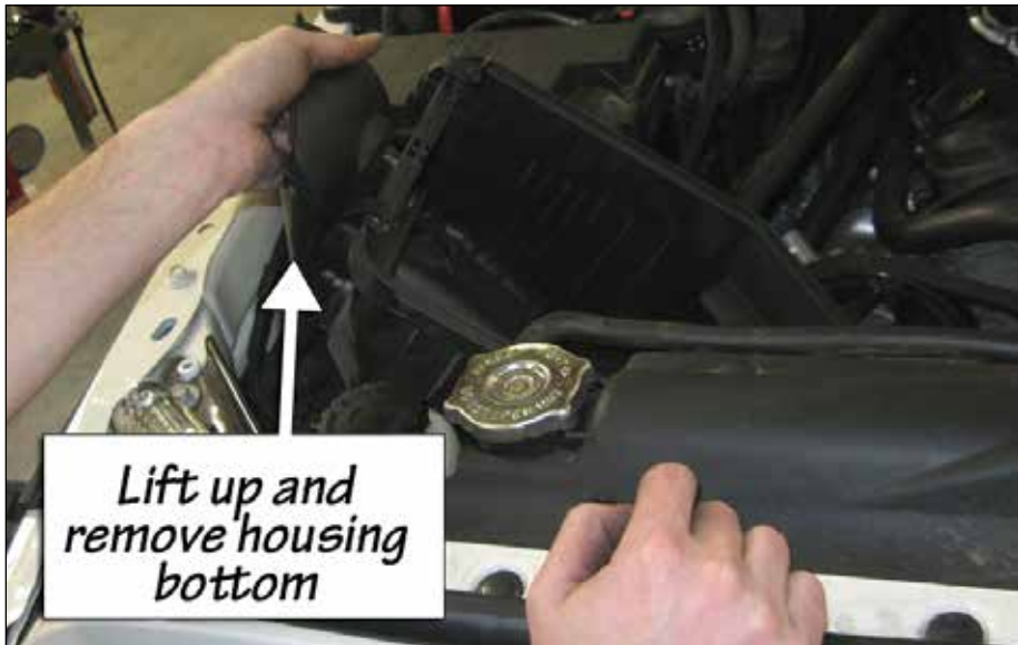
Figure 4- Removal of filter housing bottom
