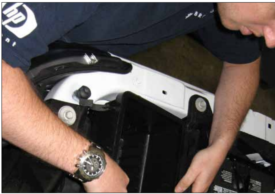
Figure 7- Removal of the stock air filter housing
