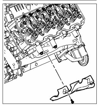
Remove the exhaust manifold bolts and nuts in the proper sequence.
