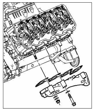
Install the BD High Flow exhaust manifold with gasket.
