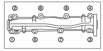
Install the exhaust manifold heat shield.
