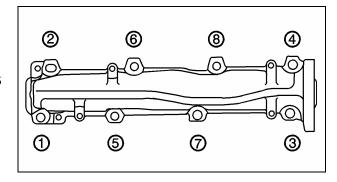
Remove the exhaust manifold.
