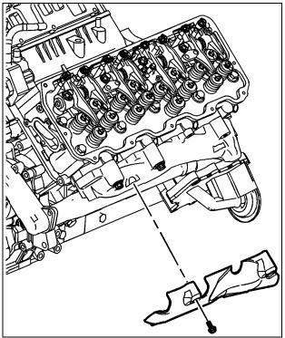
Install the exhaust pipe gasket. Align the tab on the gasket to face outward.
