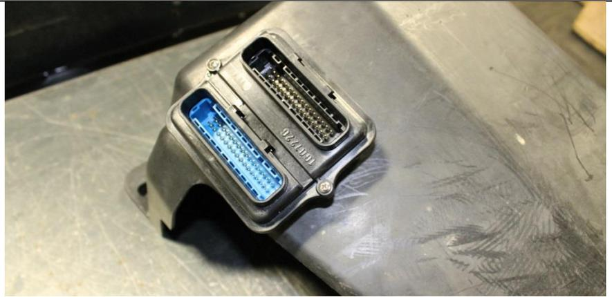
23. Connect the vehicles harness with the BLUE connector and the BD harness with the BLACK connector to the BD Tap Shifter control module.
