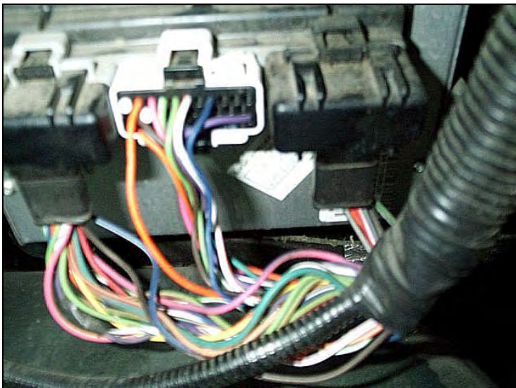
Isolate wire and install resistor. Resistor can be installed either way.
