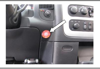
9. Using the decal as a drill template you can now drill a 1/4 hole for the main part of the switch and a 1/16 hole for the locator nub.
