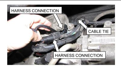
6. Remove lower dash panel and route switch harness from steering column area through grommet in firewall and connect into module harness.
